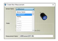
For ultrasound measurements, UAS3 gives you the option to choose either Static or Dynamic and for temperature measurements you can set the measurement interval and the emissivity.
