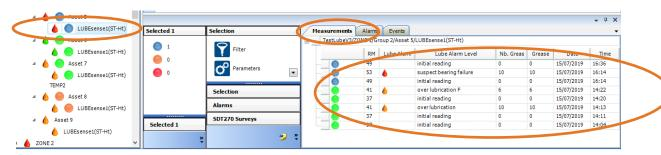
This view gives many different information sets. You can customize your view in the Parameters Menu. In the view displayed in the above screenshot, we see Alarm Level, RMS value for each measurement, Lube Alarm Status, Lube Alarm Level Specified, Number of Shots Added, Quantity of Added Grease in Grams (oz), Date and Time.
