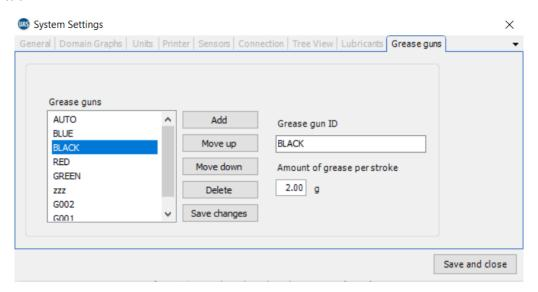
When done, left click on ADD. You can sort your list by selecting any grease gun and moving it UP or DOWN with the move up/move down buttons. You can also Edit grease gun IDs or delete them altogether. Left click Save to save your changes or the "X" in the top right to exit without saving.
