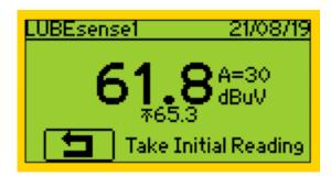
Once the reading has been taken, LUBExpert provides a screen with measurement results, representing RMS, maxRMS, PEAK and Crest Factor:
