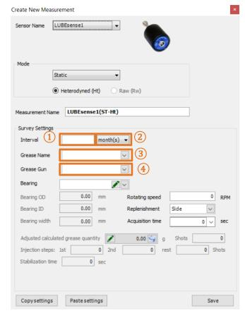
"Create New Measurement" dialogue box open, here you select the grease type for this bearing using the drop-down box beside the field Grease Name 3.
