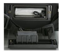
Proceed in the reverse order to remove the battery. Remove the connector by slightly pulling the 2 conductors. It should come off easily. In case of abnormal resistance, do not force and call the aftersales department.
