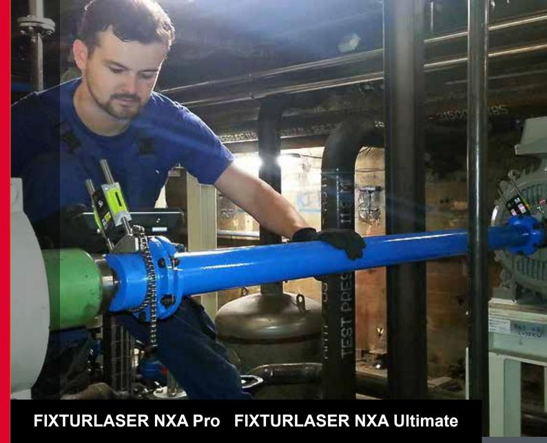
Shaft Alignment with Geometric Measurements
