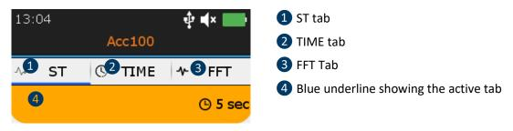
Figure 12-3 Condition indicator, time signal and spectrum tabs
