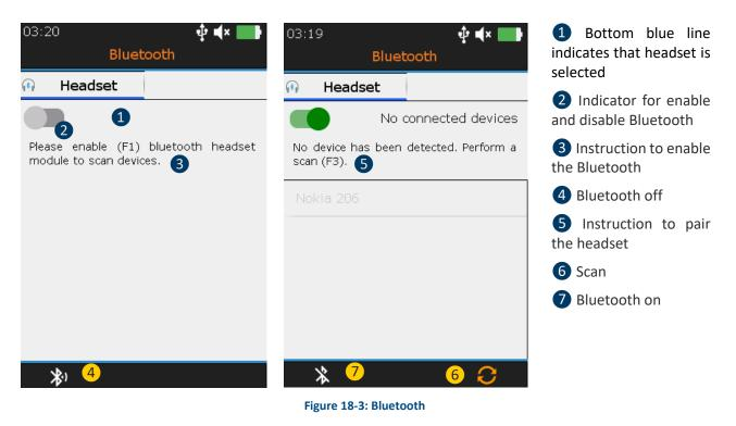
Press F1 (2) to enable the Bluetooth headset module. Switch on the headset. The headset must emit a blue flashing light. Press F3 to pair (6) the SDT340 with the headset.
