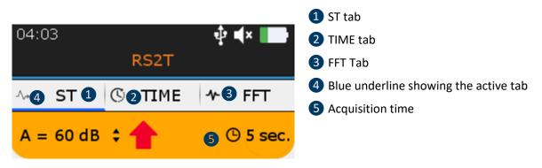
Figure 10-3 Condition indicator, time signal and spectrum tabs
