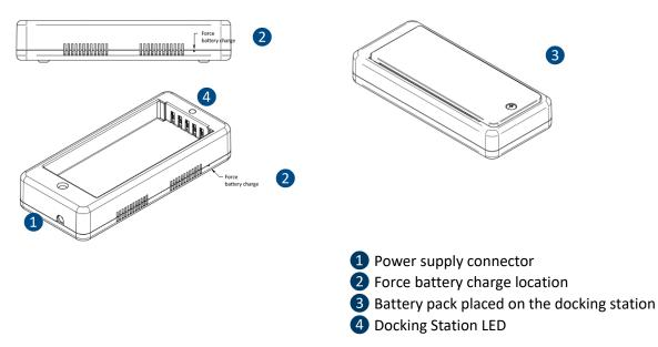
Figure 6-1 Recharge the battery
