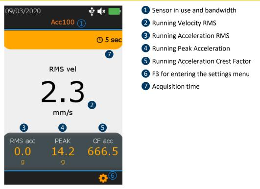
Figure 12-1 Vibration measurement screen
