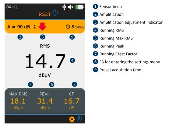
Figure 10-1 Ultrasound measurement screen
