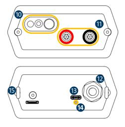
10 Tachometer, laser and IR thermometer
