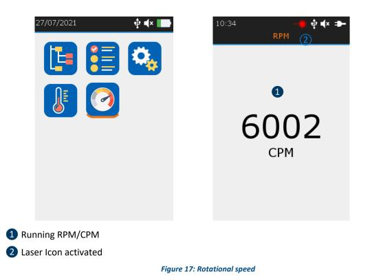
From the **Home** screen, select the RPM icon and press **Enter**. The running RPM screen is displayed (Figure 17). The value **1** is refreshed twice per seconds (500 ms). Press the **Laser** hold-on key to activate it. The laser icon **2** indicates when the laser is on.
