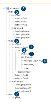
Unit 1 5, Unit 2 6 and Unit 3 7 are the children of My Factory 8. They have the same level in the tree structure. In the same way, Centrifugal pump 1, 2 and 3 are children of Pump group and have the same level. Fan group is the parent of Belt Drive fan 1, 2 and 3...
