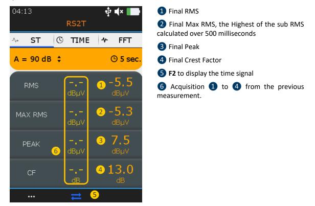
Figure 11-1 Ultrasound ST tab
