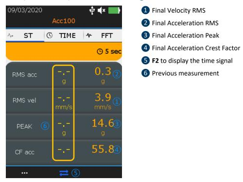
Figure 13-1 Vibration ST tab
